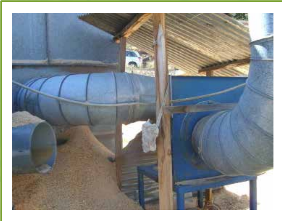
Fan working in a dust extraction system in a sawmill
