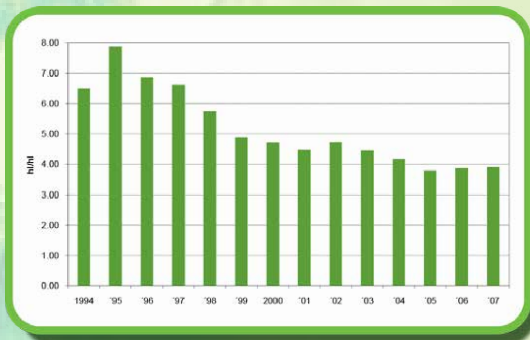
Figure 8: Specific water consumption of a brewery.
