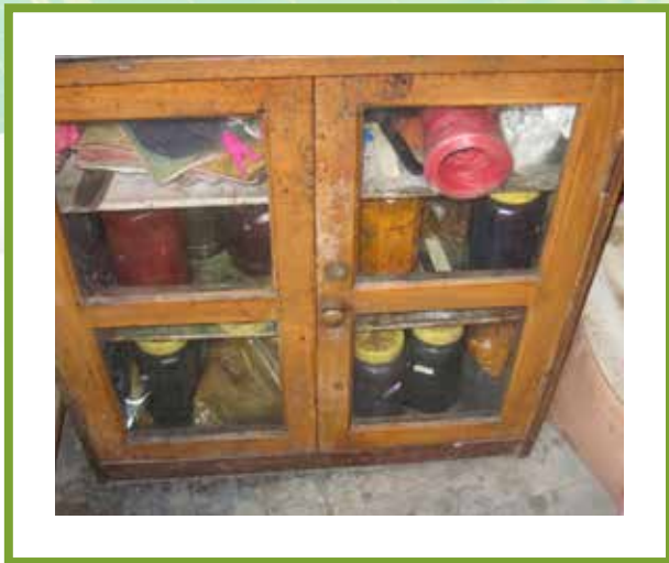
Storage of chemicals in cupboard without labelling
