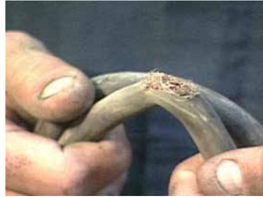
Wire with damaged insulation can cause electric shock
