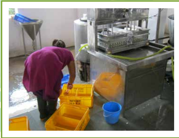
Use of water via hose pipe without flow controller which causes wastage of water.
