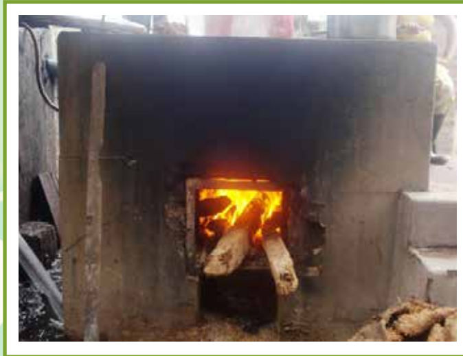
Slight improvement in burning chambers firewood feeder section. The Net is installed for firewood and ash is collected below.
