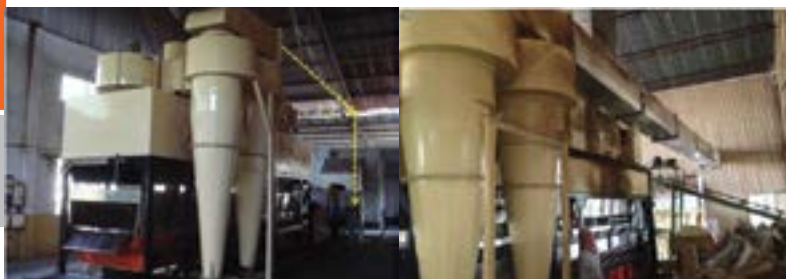
Waste heat from the dryer is reused to heat up the secondary intake air for the furnace
