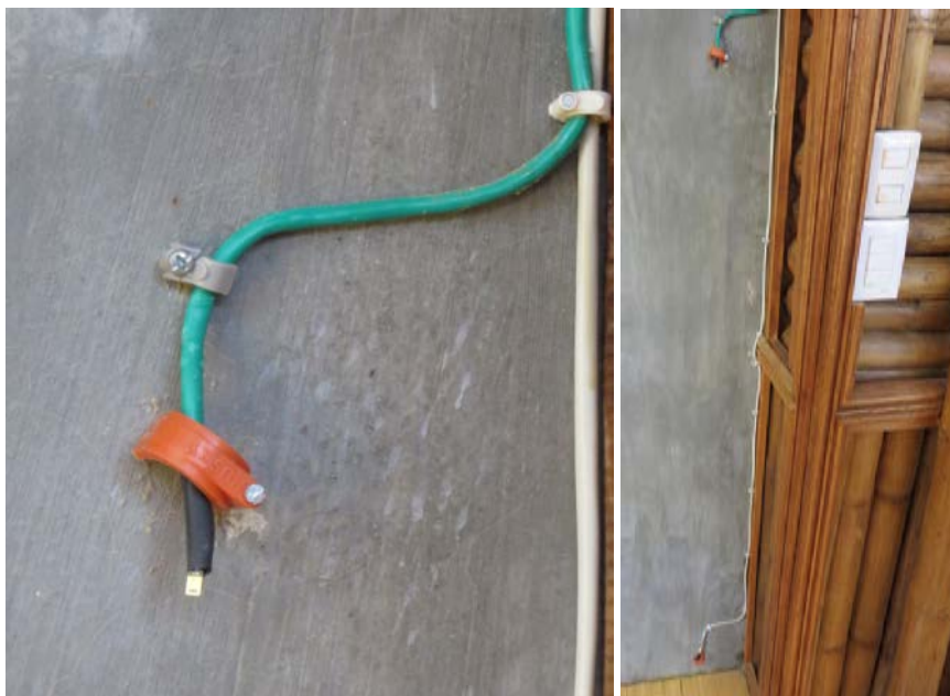
Figure 12: Sensirion SHT75 sensor mounted on the wall
